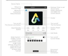
After Bluetooth connection, the device immediately switches to Bluetooth mode.
